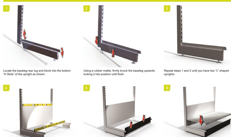
Connect both "L" shaped uprights together by fitting a back panel into the bottom "H" slots of the uprights. Now check levels are correct by adjusting the foot discs as required. Fit the plinth skirting into position by slotting it between the front capping on the baselegs. Fit the base shelf onto the baseleg runners. Now fit all remaining back panels.
